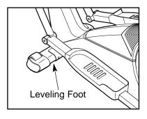
rocks slightly during use, turn one or both of the leveling feet under the front stabiliser until the rocking motion is eliminated.
